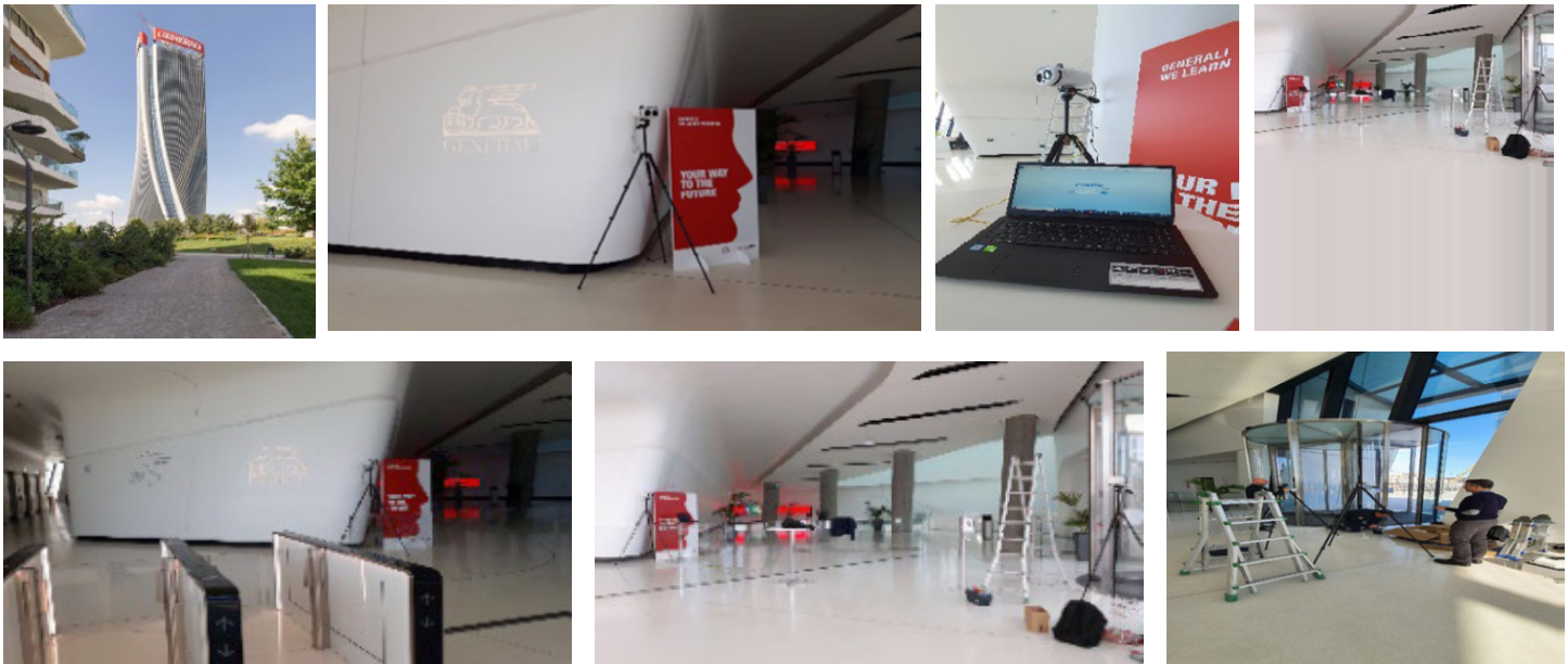
6 kits were installed to monitor the temperature of the people walking into a large commercial building.
